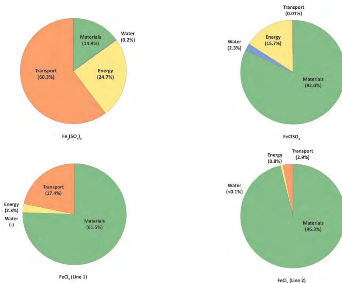
Figure D-1: Contribution of impacts on the carbon footprint of iron-based coagulants
