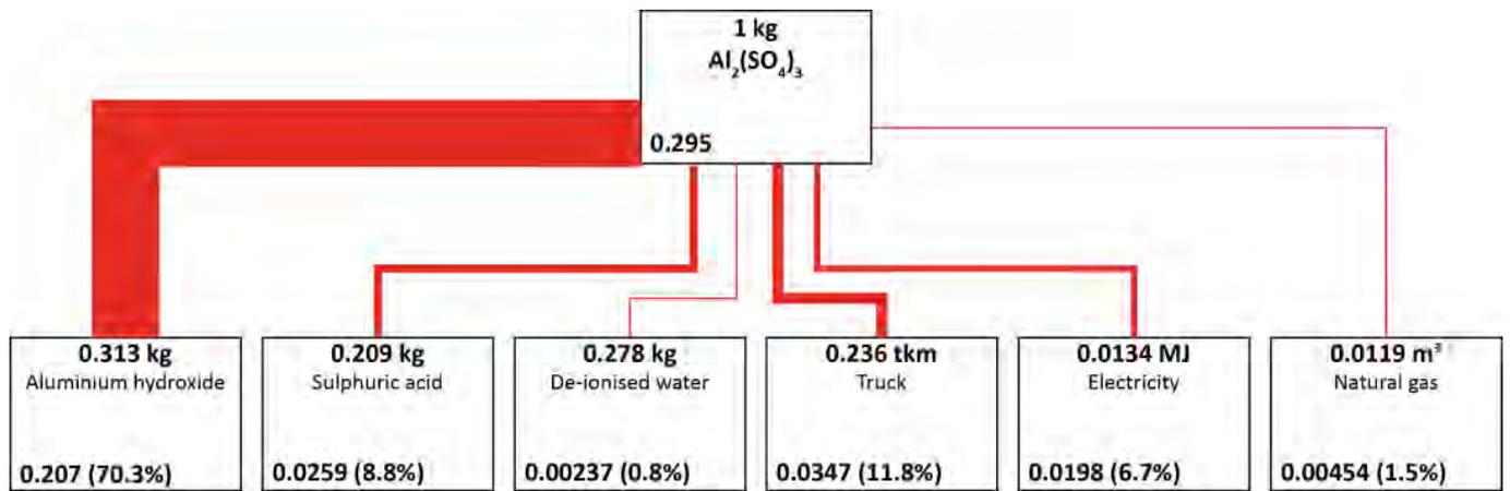
Figure C-3: Overview of the  $Al_2(SO_4)_3$  17%  $Al_2O_3$  (solid) production process tree
