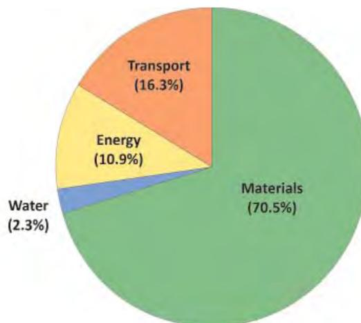
Figure A-2: Contribution of impacts on the carbon footprint of different coagulants
