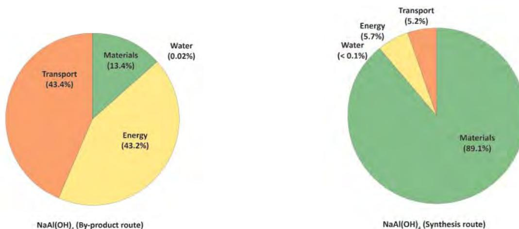
Figure E-1: Contribution of impacts on the carbon footprint of sodium aluminate coagulants
