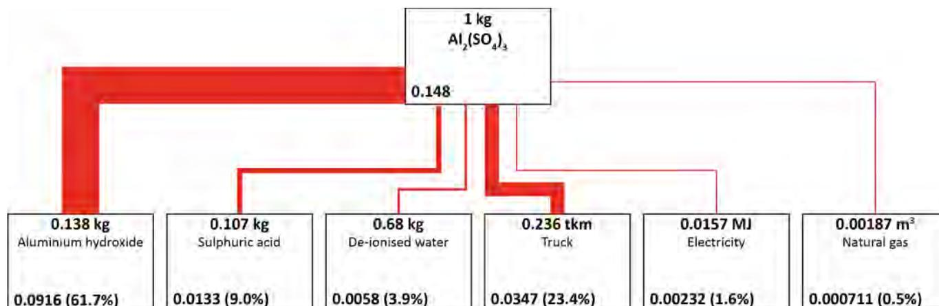
Figure C-2: Overview of the Al<sub>2</sub>(SO<sub>4</sub>)<sub>3</sub> 8.25% Al<sub>2</sub>O<sub>3</sub> (liquid) production process tree
