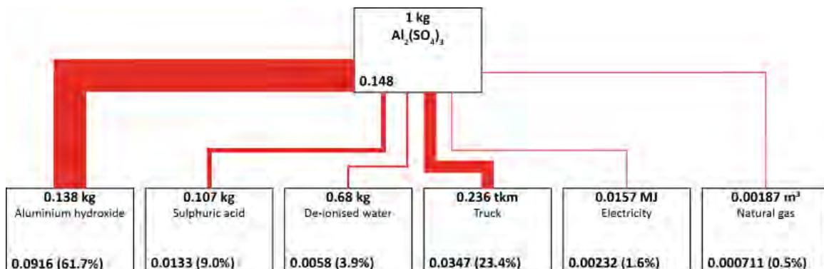
Figure 1: Tree diagram showing overview of process flows and emissions for Al<sub>2</sub>(SO<sub>4</sub>)<sub>3</sub>
