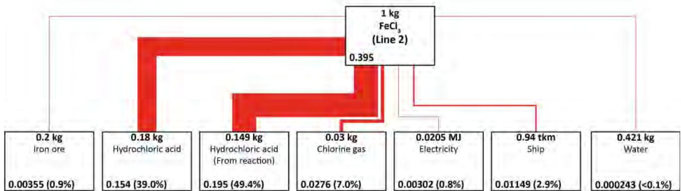
Figure D-5: Overview of the FeCl<sub>3</sub> (iron oxide) production process tree
