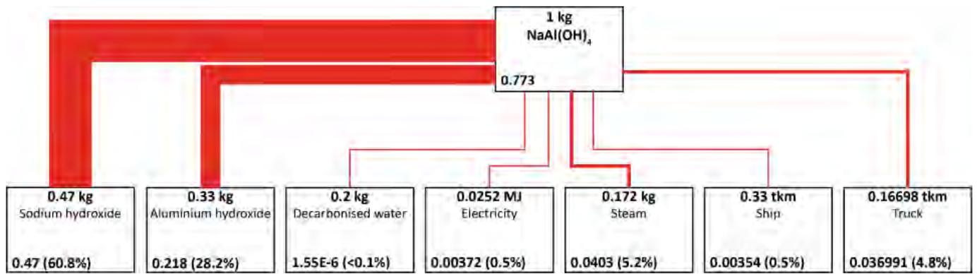
Figure E-3: Overview of the  $\text{NaAl(OH)}_4$  (synthesis route) production process tree
