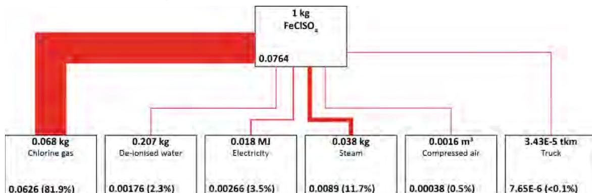
Figure D-3: Overview of the FeClSO<sub>4</sub> production process tree
