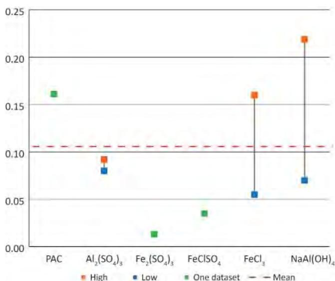
Figure A-1: Range of carbon footprint values for coagulants investigated (kg CO<sub>2</sub>-eq/mole Fe<sup>3+</sup> or Al<sup>3+</sup>)
