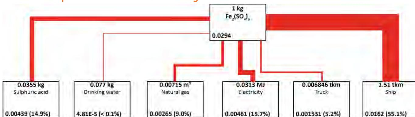
Figure D-2: Overview of the Fe<sub>2</sub>(SO<sub>4</sub>)<sub>3</sub> production process tree
